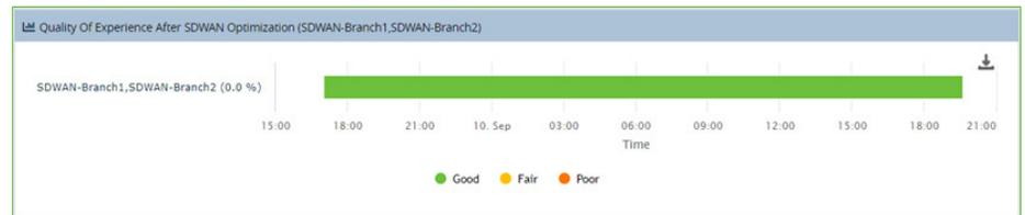
The quality of experience with SDWAN resulting from traffic steering, Forward Error Correction (FEC), replication
